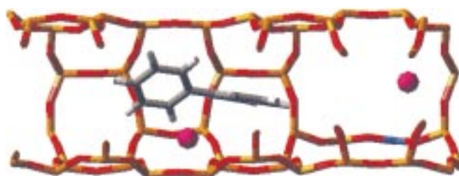
Figure 1. Cross-sectional view of biphenyl ( BP, S_0 ) occluded in the straight channel of Na_4Si_{92}Al_4O_{192} zeolite perpendicular to the b axis. The yellow Si, blue Al, and red O cylinders represent the ZSM-5 framework, the pink balls represent the extra-framework Na^+ cations, the shaded and white cylinders represent the C and H atoms of BP, respectively.
